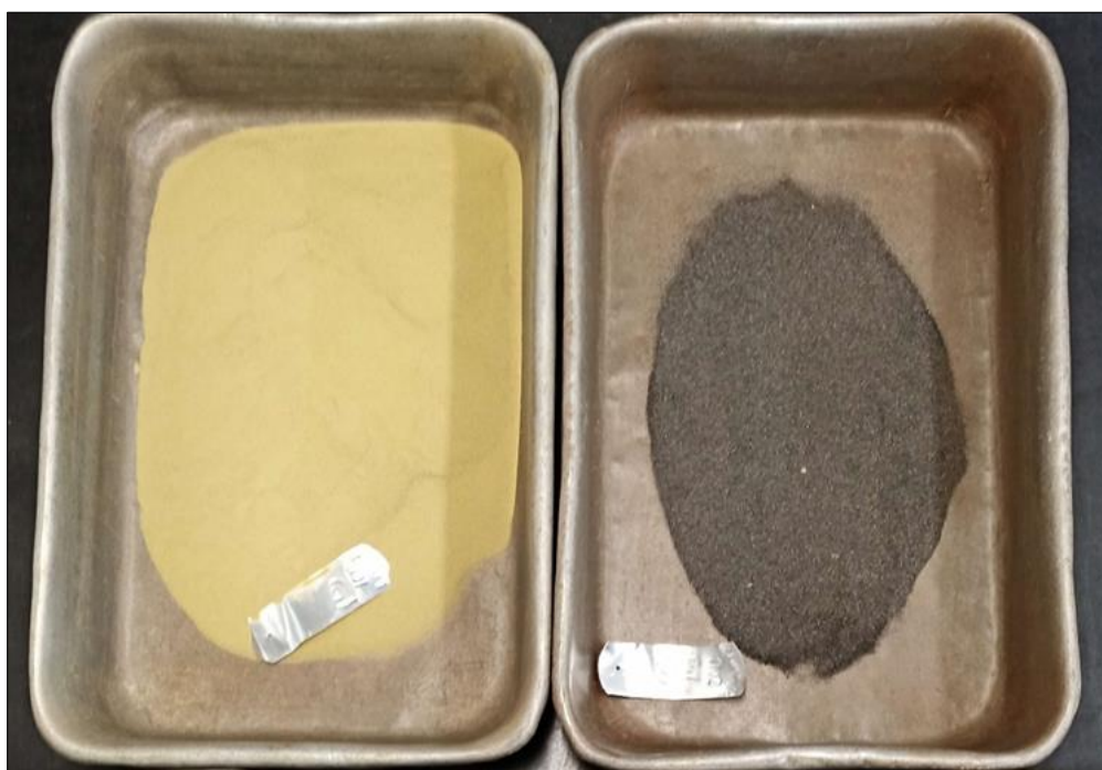
Figure 1: Rare earth (LHS) and HMC (RHS) streams from wet shaking table tests after flotation
